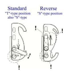
Comparison "Standard" and "Reverse" position of the needle thread take-up.
