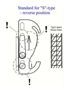
In reverse position and with S-type needle plate, we achieve the tight seam.
